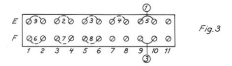
Note If an extension in each group is to be priority connected, it must be remembered that every strapped units digit provides a priority-marked extension within each extension group.
